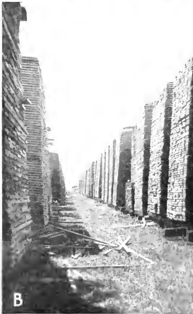
Rear alleys; bad and good practice: A, Poor piling of yard lumber. Overhanging ends, inadequate stickering, insufficient and improper foundations, weeds, and a narrow and obstructed alley all cause degrade, with its resulting loss; B, an adequate rear alley, wide and well-kept except for the few scattered stickers. All the piles are set up properly (box piled), and the sanitation is good; C, one side of a well-appearing rear alley. The stock is piled without overhanging ends (box piling), a desirable feature. Three or four rear pile ends, in addition, have drip boards. On the other hand, higher foundations are desirable.
